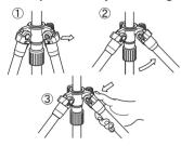
To change the angle of each leg, close the leg slightly, and then pull the leg angle adjustment lock out. There is a choice of two other angle positions. After choosing the desired leg angle, securely push in the adjustment lock.
