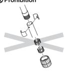
Do not remove the nut and take out pieces. If it has been removed, insert the pieces as per the above specification.
