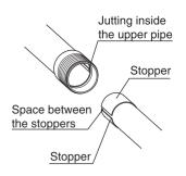
Match the space between the stoppers and jutting inside the upper pipe when the pipe is connecting.
