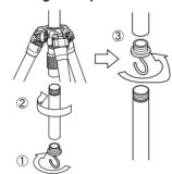
Remove the center column base stopper, and then remove the lower part of center column.
