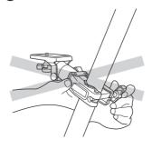
Please do not use an optional clamp head for a carbon fiber tripod. The pipe may be damaged.
