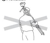
The hanging weight shall be a part of the maximum loading capacity.
