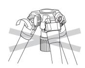
Do not turn the center column stopper while pulling out the center column. The internal parts may be damaged.
